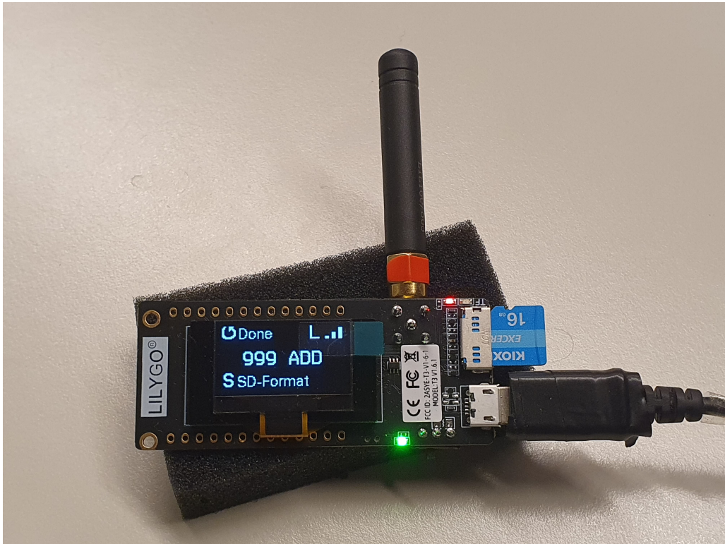
Figure 3.8: Overview of the OLED Status and Number output
