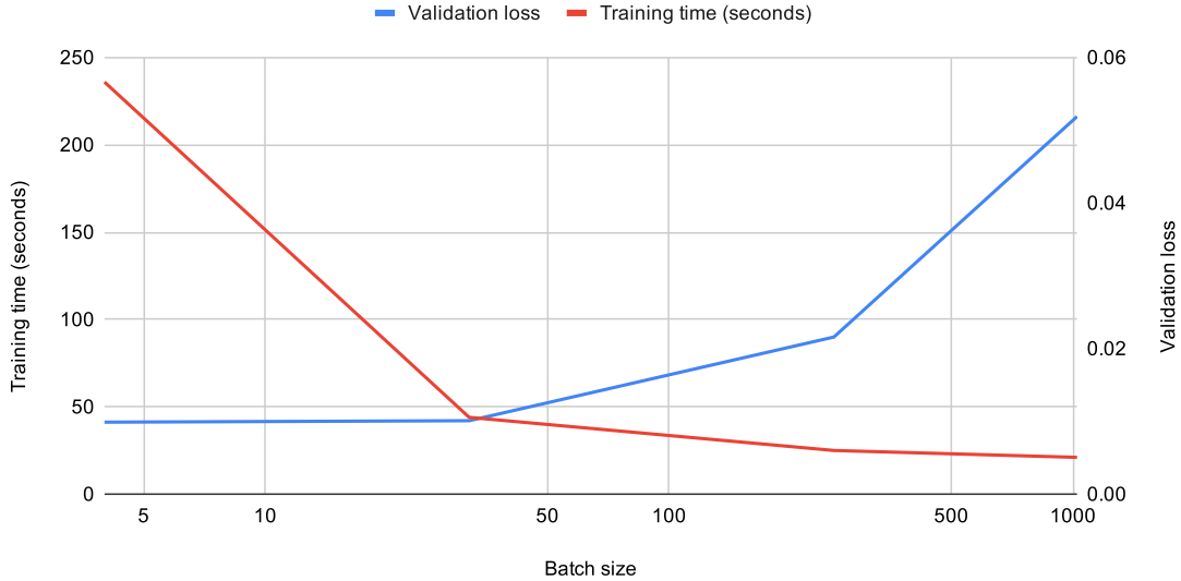
Figure 10: Influence of batch size on training convergence (for unsupervised learning with CCE loss function, 50 epochs). This figure was generated from the values in Table 4.
