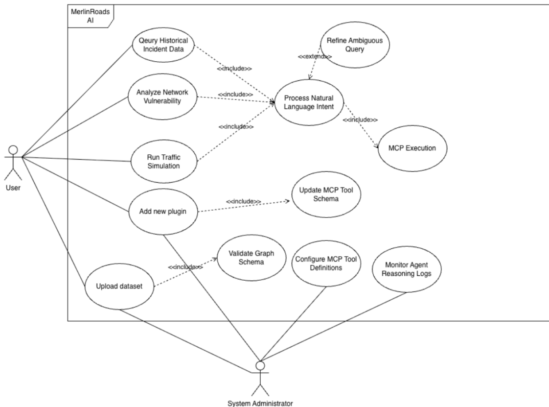
Figure D.1: Use case diagram for MerlinRoads AI, showing the User and System Administrator actors and their associated use cases.
